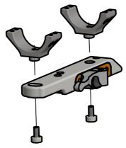
**3 - LOCK THE RINGS** lock the rings using a scope or a ground cylinder to ensure the perfect lineup of the rings
