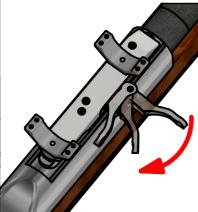
**6 -** Position the scope, **SCREW THE TOP RINGS** with the provided screws at their specific bases
